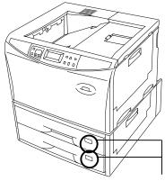
The size indicator plate on the front of the paper feed cassettes is illuminated by LED. This LED indicates the status of the cassettes as follows depending on whether it is on, off or flashing.
